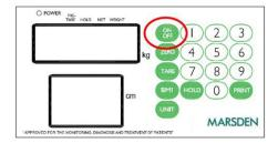
Press the ON/OFF button when the scale is turned on. The scale will now power down.
